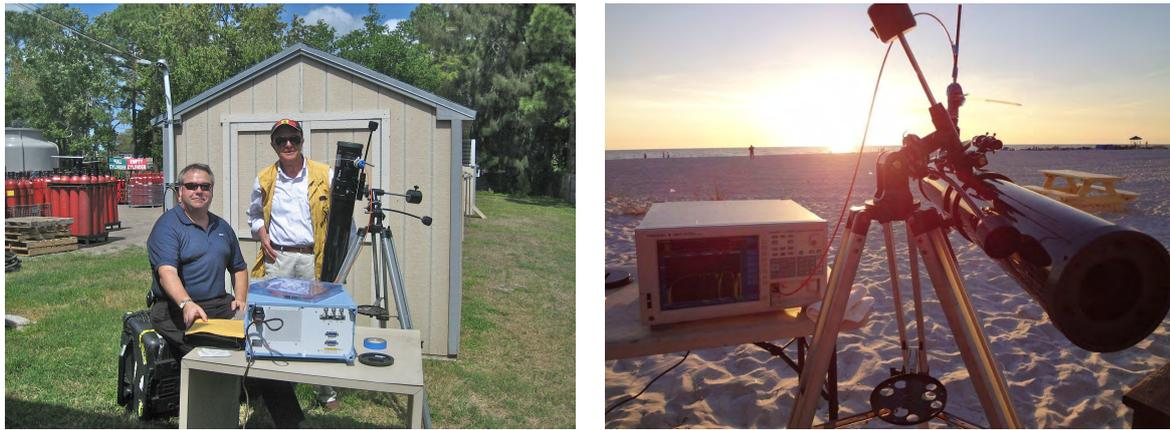
Fig. 13. The experimental set up for the scan of Sunlight from the Zenith to the horizon used in Ref. [14] comprising a conventional refraction telescope with a Yokogawa wavelength analyzer directly connected to the eyepiece. The top picture shows the the calibration of the instrument by a manufacturer representative for scans of the Sun at the Zenith, and the position of the instrument at sunset.
