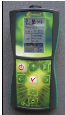
Fig. 2. The Kiwi-Meter, a portable, non-destructive vis/NIR device used to measure the DAindex™ and to follow the fruit ripening of the fruits when attached to the vine.
