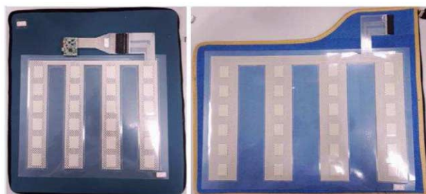
Fig. 13. Types of contact sensor: cushion (left), pedal mat (right).
