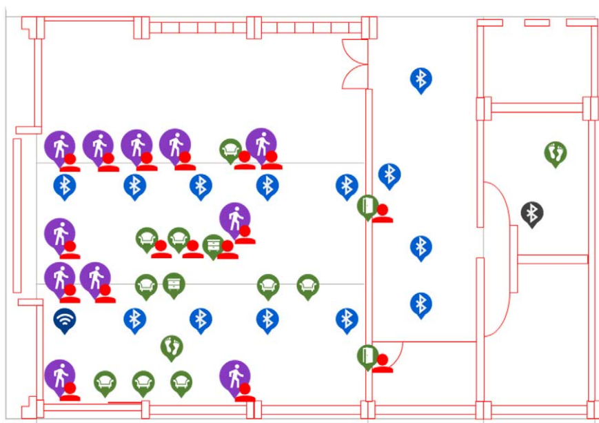
Fig. 19. The web monitoring of the location of the personnel.
