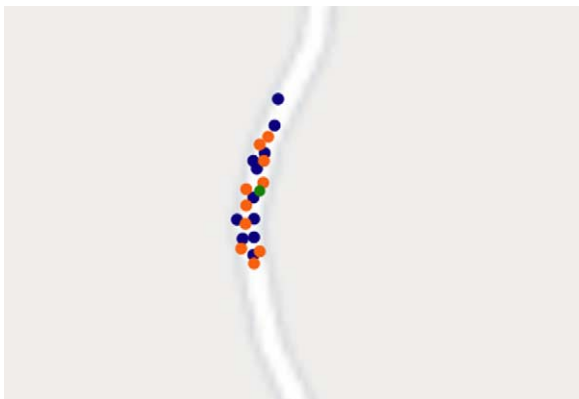
Fig. 11. Location of all the OSLSPs generated during the experiment around obstacle o_8 . The true obstacle location is shown as a green point. The points with the same color (blue or orange) are the OSLSPs from a particular cyclist.
