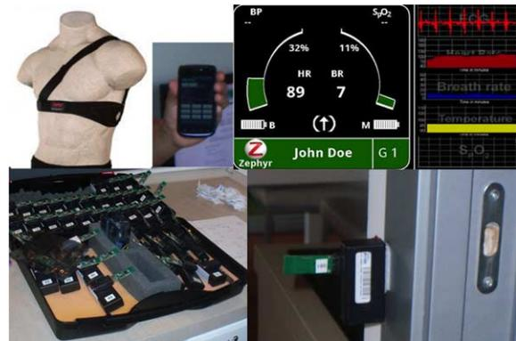
Fig. 11. Devices used by CMU and Utah Universities. Top image shows the chest strap and android mobile wore by our actor. Down at left the case where the radio beacons are stored can be seen. Down at right a detail where a radio was placed in a door.
