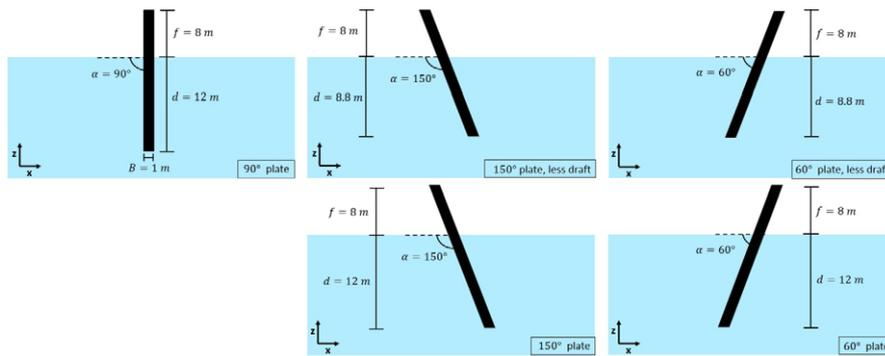
Fig. 2. Five tested breakwater models and their particulars.
