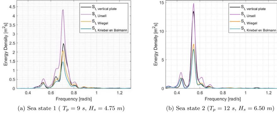
Fig. 4. Transmitted spectra compared with theoretical models.
