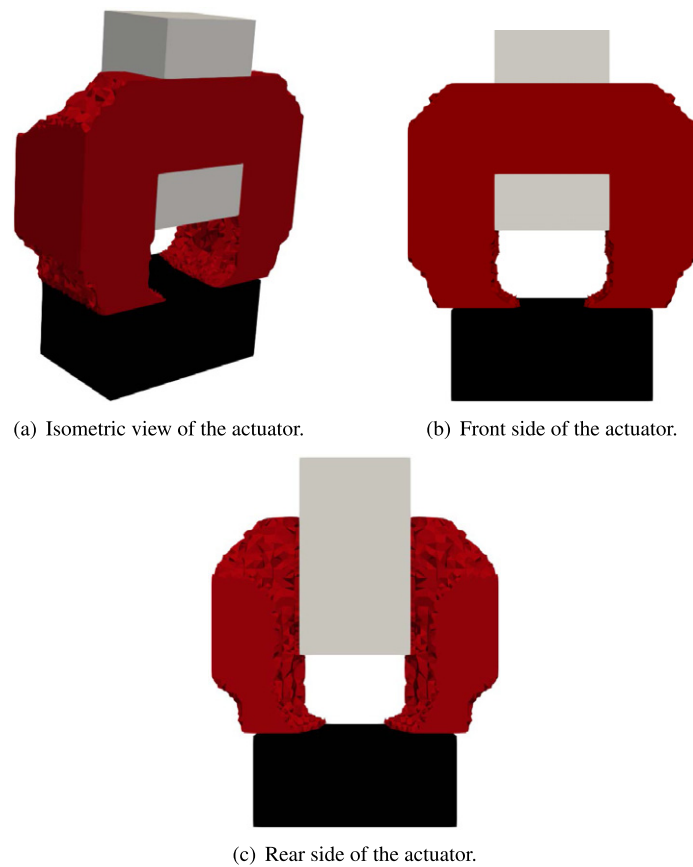
Fig. 12. Optimized 3D geometry, assuming a linear material behaviour for yoke and anchor. Interface conditions are fulfilled by the use of edge elements. Non-conforming interfaces are used in the air gap between yoke and anchor. The air gap distance between yoke and anchor is 1 mm.
