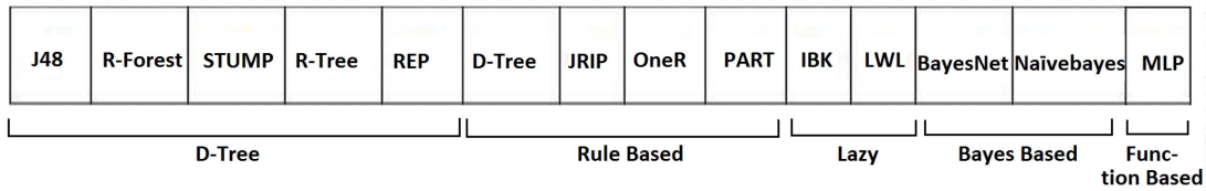
Fig. 4. The chromosome of each individual as used by the genetic algorithm. It is partitioned into five classifier families, including Decision tree, Rule based, Lazy, Bayes based and Function based. Each gene expresses whether or not the respective individual classifier is part of the classifier combination.
