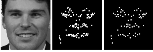
Fig. 5. Example of original image, fiducial points detected by Gabor wavelets and clustered points (64 clusters) using Face Specific Position approach (left to right).
