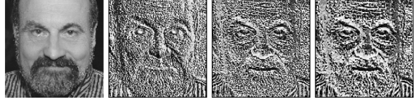
Fig. 4. An example of the original image and the LBP image after applying the original LBP , LBP_{8,1} and LBP_{8,2} operators.
