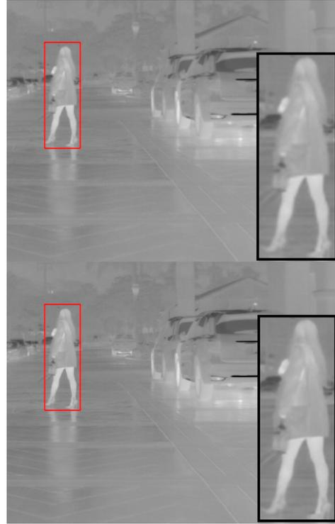
Fig. 6. Super resolution applied on thermal images. Top: bicubic interpolation. Bottom: SR  $\times 2$ .
