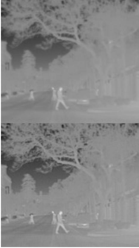
Fig. 5. Unsharp masking. Top: initial thermal image  $f$ , bottom: de-blurred image  $f_1$ .
