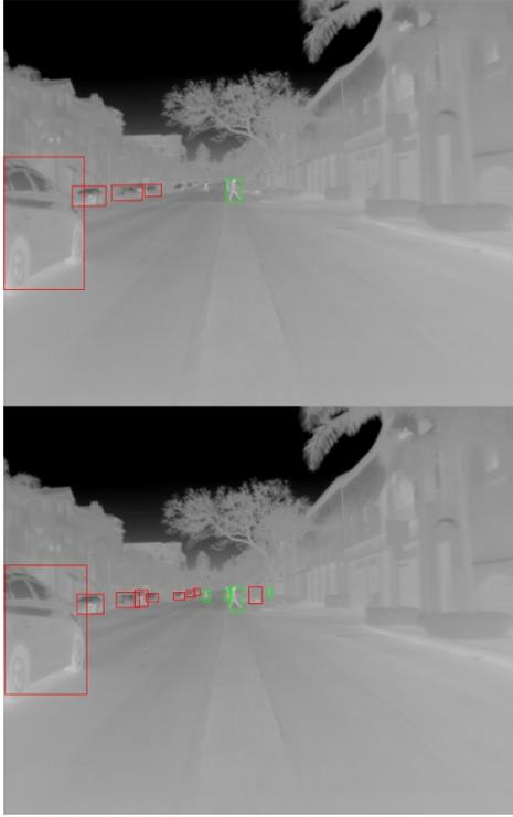
Fig. 8. Comparison between FLIR annotation (top) and the new one (bottom). Red boxes are labeled cars, Green boxes are labeled pedestrians.
