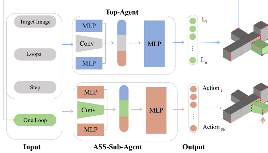
Fig. 5. The triple can be the input of top-agent, which will output an option related with loop index. The features of the loop as the augmentation of state are inputted into ASS-Sub-Agent, which decides how to operate on this loop.
