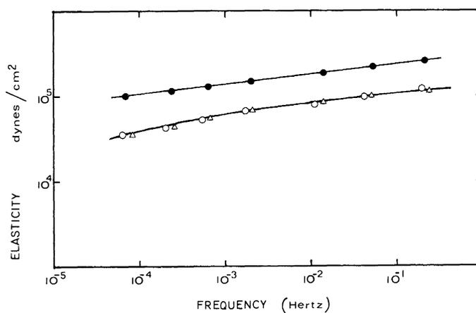
Fig. 10. Comparative elastic modulus data of surface layers of 0.4 per cent solution of fibrinogen from sheep (-●-), bovine (-o-), and human (-△-) origins.
