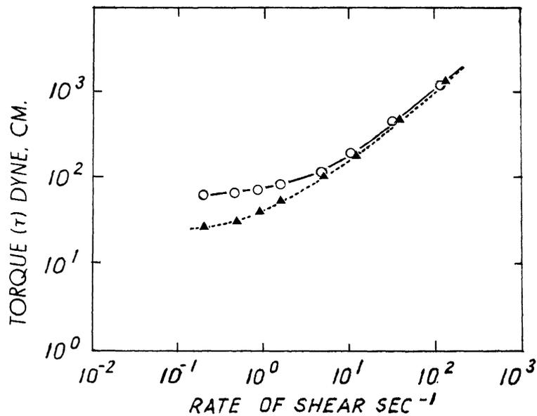
Fig. 16. A comparison of viscous resistance or torque values between the surface layers of a platelet-rich human plasma containing 2% red blood cells and the surface layers of the same plasma without the red blood cells. —○— Platelet-rich plasma; —▲— 2% red blood cells in platelet-rich plasma.
