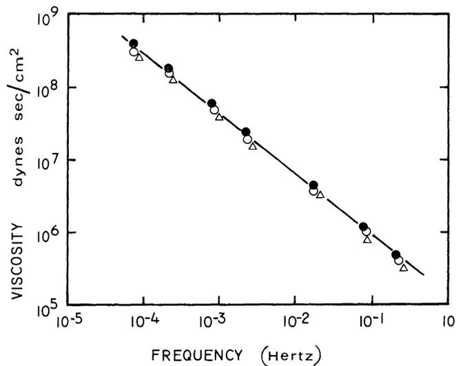
Fig. 9. Plot of viscosity (dynes. sec/cm<sup>2</sup>) versus frequency of 0.4 per cent solutions of fibrinogen from sheep (-●-), bovine (-o-), and human (-△-) origins.
