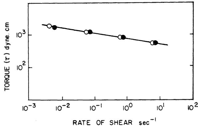
Fig. 8. A comparison of torque values, secured from surface layers of a 0.4 per cent human fibrinogen solution, formed at (-●-) oil-fibrinogen and (-o-) air-fibrinogen interfaces.
