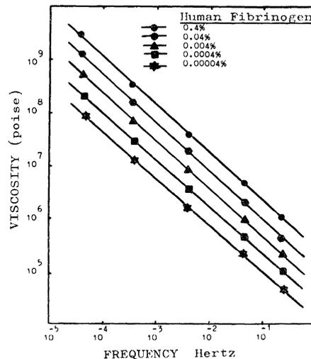
Fig. 11. Viscosity of surface layers of varying concentrations of highly purified human fibrinogen versus frequency.
