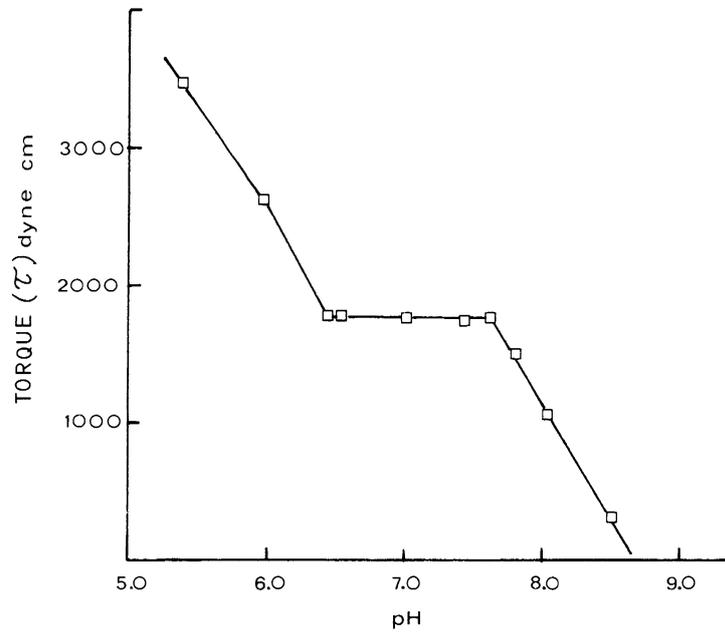
Fig. 20. The effect of pH on the rigidity of surface layers of highly purified human fibrinogen solutions employing tris-maleate buffers.
