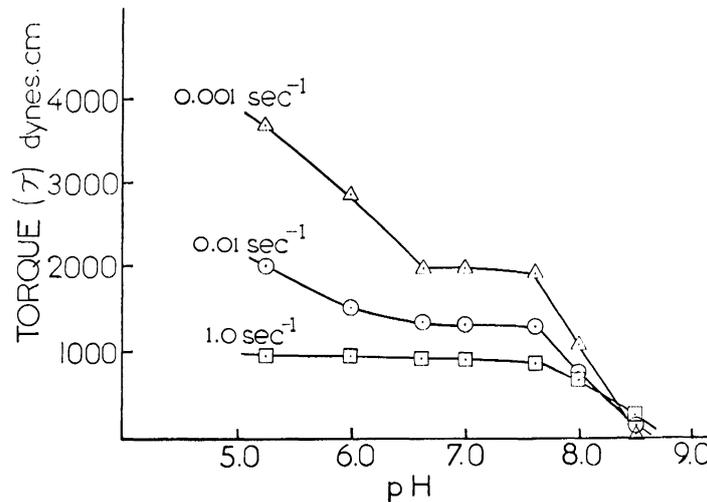
Fig. 22. Comparison of rigidity values of surface layers of 0.4% fibrinogen at varying pH and at shear rates varying from 0.001 to 1.0 sec<sup>-1</sup> employing tris-maleate buffers.
