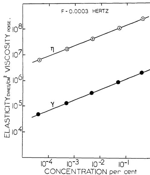
Fig. 13. Comparisons of viscosities ( $\eta$ ) and elasticities ( $\gamma$ ) plotted against different concentrations of human fibrinogen at frequency  $F = 0.0003$  Hertz.
