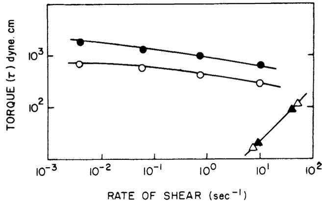
Fig. 24. Comparisons of torque values from surface layers between 0.4% fibrinogen solution and 0.25% highly purified  $\beta$ -lipoprotein added to the 0.4% fibrinogen solution with and without preshearing at 1000 sec<sup>-1</sup>. ●-Fibrinogen after pre-shear, ○-fibrinogen without pre-shear, ▲-fibrinogen plus  $\beta$ -lipoprotein after pre-shear, △-fibrinogen plus  $\beta$ -lipoprotein without pre-shear.
