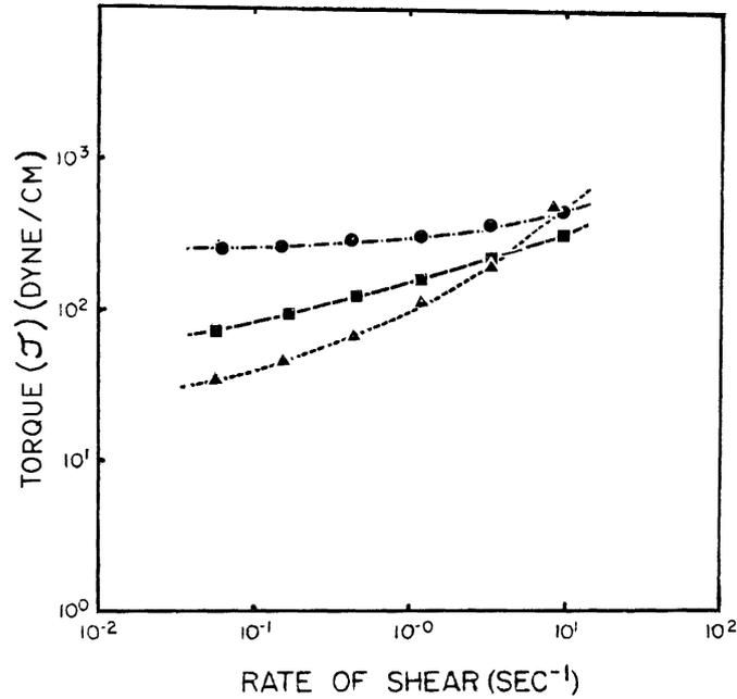
Fig. 15. Torque ( $\mathcal{J}$ ) measurements of —●— 0.4% fibrinogen solution; —■— 10% red blood cell suspension in 0.4% fibrinogen solution; —▲— 43% red blood cell suspension in 0.4% fibrinogen solution.
