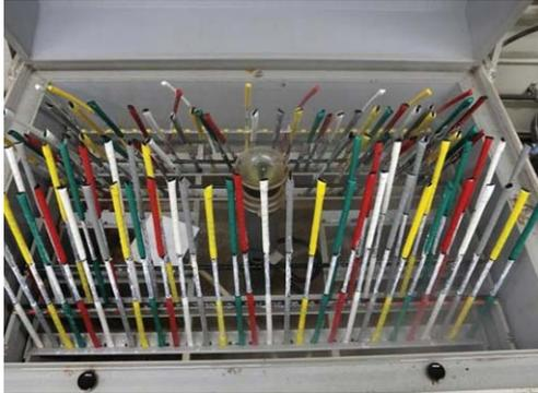
Fig. 2. Salt spray test.
