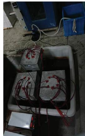
Fig. 4. Experimental device of drying-wetting cycle and chloride ion corrosion.
