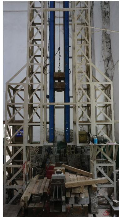
Fig. 5. Drop hammer impact test setup.
