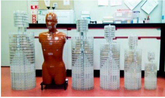
Fig. 1. Use five tissue-equivalent and Rando phantoms as patient surrogates.
