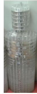
Fig. 2. Illustration of the 70-kg phantom with the TLD measurement positions marked.
