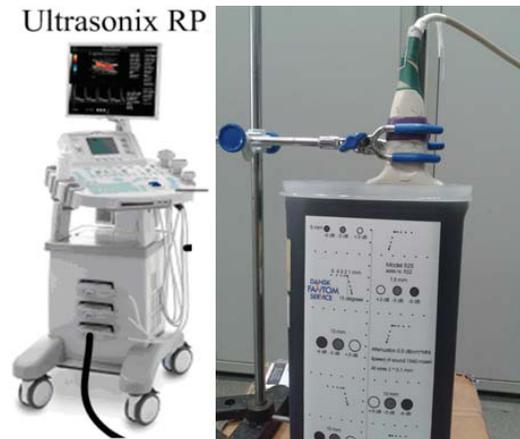
Fig. 5. The overview of the experimental setup. The linear transducer of the commercial Ultrasonix RP ultrasound system was chosen to scan the target phantom (No: 922, model 525).
