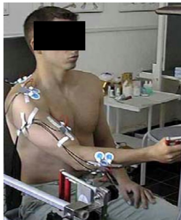
Fig. 2. Upper limb location. The arm is flexed at an angle of 45^\circ . The angle between the arm and forearm is set to 135^\circ and there is supination of the forearm at 30^\circ . The wrist is in a neutral position. There is no abduction or rotation in the arm.
