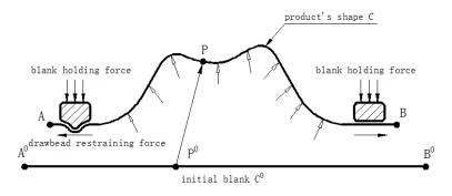
Fig. 1. Schematic view of FE approach on one step inverse forming.
