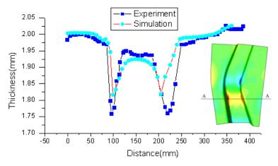
Fig. 5. The comparison value between experiment and simulation on section A-A.
