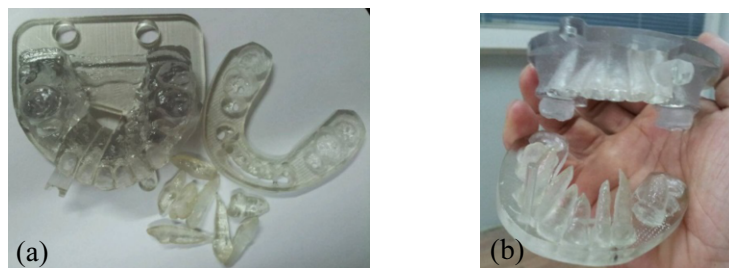
Fig. 5. Fabricated models (a) fabricated models and guide by 3D printing; (b) teeth in guide and maxilla.
