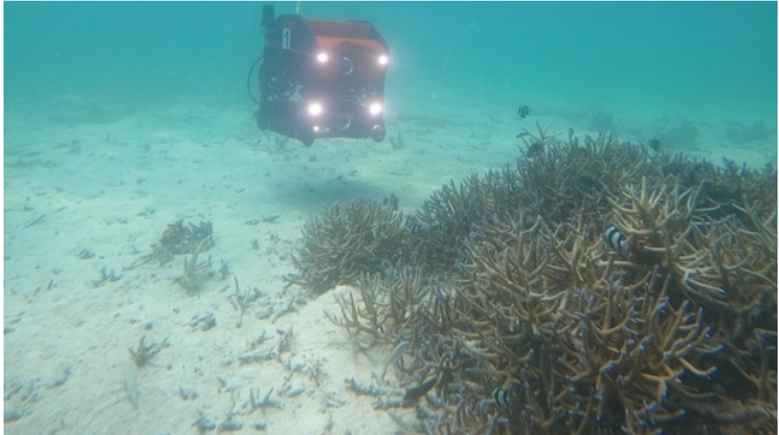
The ROV in use during initial tests to record coral reef imagery in shallow waters. (Photo credit: Raheem D.A., REEF)
