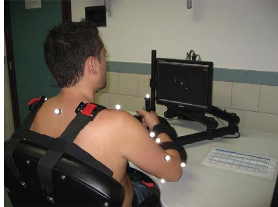
Fig. 1. Young adult participant engaged in the circle-drawing task with InMotion Arm Robot installed at the Movement Analysis and Robotics Laboratory (MARlab) of the Bambino Gesù Children's Hospital. Except for the one placed on the sternum, all the markers for the optical tracker system are showed in the figure.
