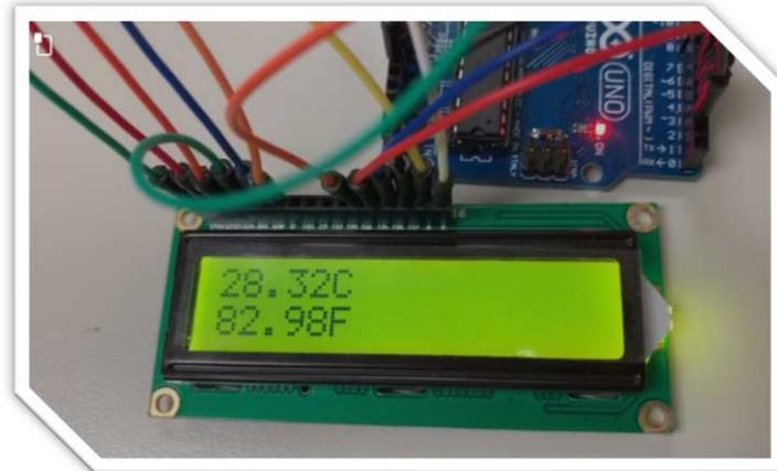
Fig. 4. Temperature sensor and Arduino board.
